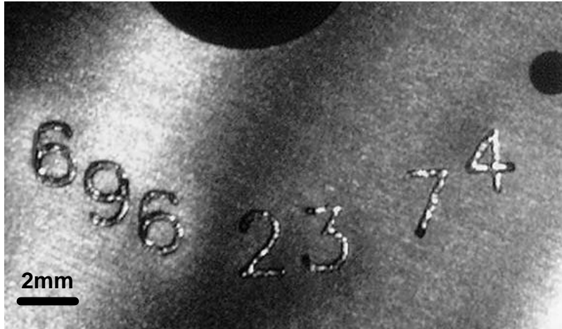
FIGURE 8. Direct Part Marking Using LENS. A Molybdenum Disk Was Marked With Stainless Steel Raised Lettering.
