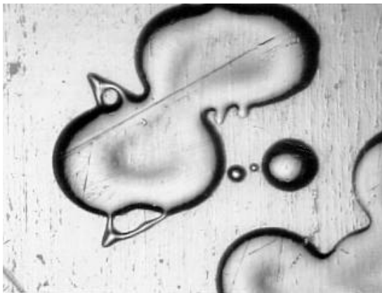
FIGURE 4. Unacceptable Ink Jet Markings
